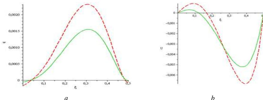
**Fig. 2. Graphs of transverse  $W_0^*$  (a) and longitudinal  $U_0^*$  (b). displacements of points of the plate at -  $z_1^* = h/2$  dashed line; -  $z_1^* = h/3$  solid line.**
