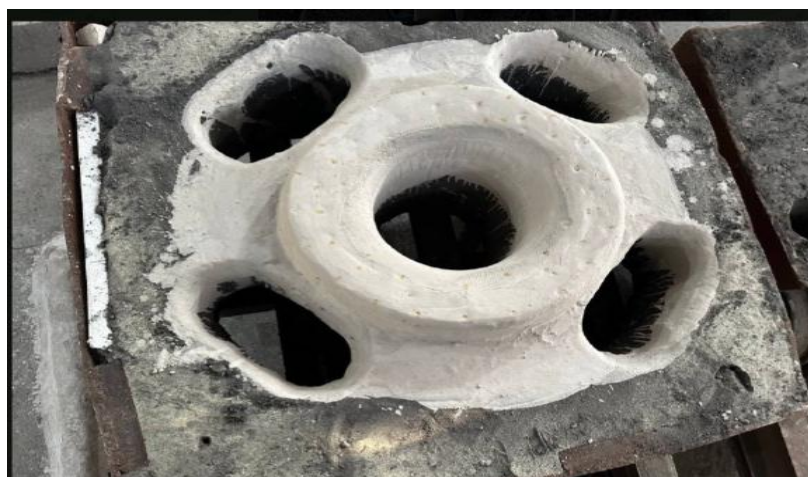
(b) Mold form made based on the model
