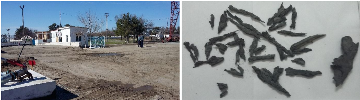
Figure 4 Samples from torn parts of the tread at turns
