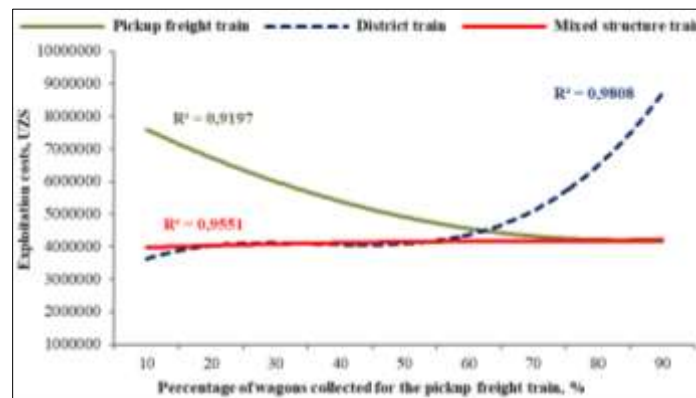
Fig. 7. Changes in exploitation costs at movement of trains under the conditions of the constant norm of the mixed-structure trains set on railway sites
