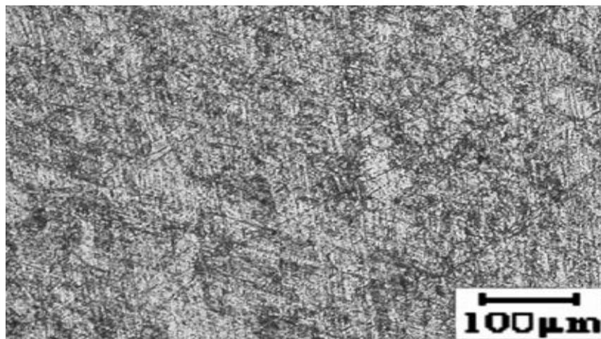
Figure 2. Microstructure of Cu-Cr alloy
