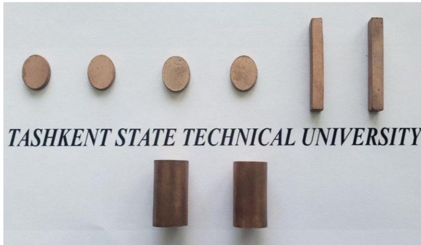
Figure1. Sample for metallographic analysis from Cu-Cr material
